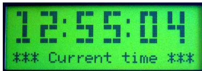
Figure 23: Shows a 4x20 line display with the time written to it using the “Write Large Number String to LCD” command and the remaining text written to it using the “Write Parsed String” command.
